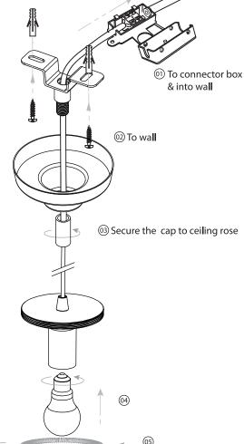
This product is not supplied with a bulb. Please use a certified E27 (E26 for US ver) bulb that lies within the suggested energy efficiency index as stated on the energy efficiency label. Any bulb used must comply with the recommended maximum voltage suggested on the safety label located on the product.
